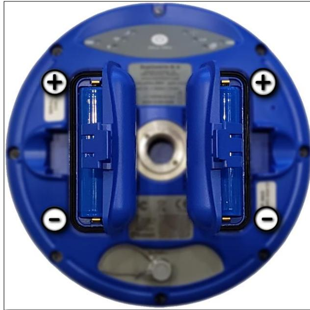
Figure 4: Battery Installation
