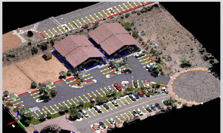
Feature Extraction of Curbs, Parking Lines, and Building Footprints
